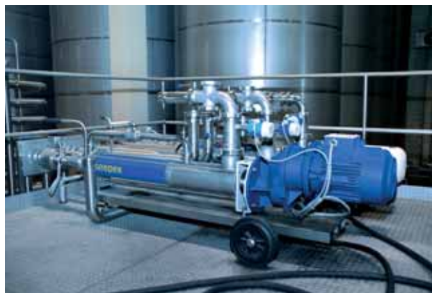
Pump of range BCSB 35-6L Conveying product: Wine Conveying capacity: 32 m 3 /h (140 GPM) Pressure: 2 bar (29 psi) • Temperature: 20 °C (68 °F)
