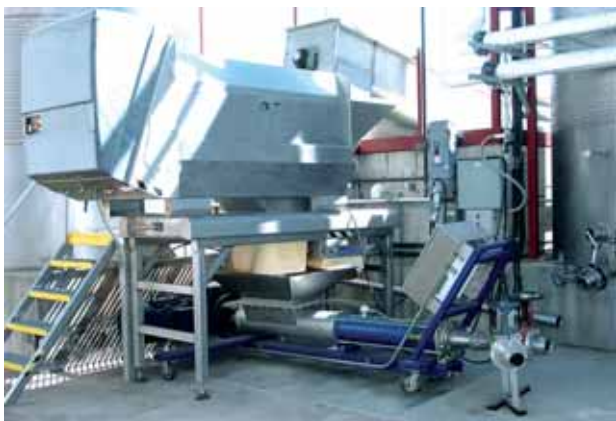
Pump of range BT 130-6L Conveying product: Mash Conveying capacity: 68 m 3 /h (300 GPM) Pressure: 4 bar (58 psi) • Temperature: 20 °C (68 °F)
