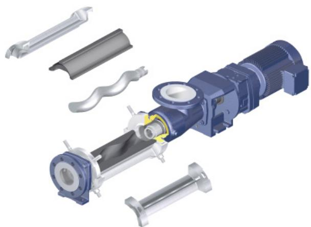
Thanks to ingenious design principles, maintenance work on the rotor and stator can be carried out with minimal effort and in the shortest of time. Compared with pumps without "Smart Conveying Technology" maintenance times to be reduced by 85 %.
